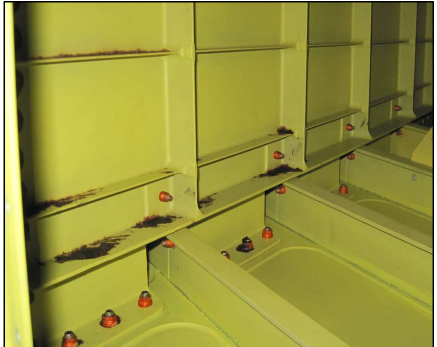
Figure 3 Areas of typical microbiological growth on a wing spar
