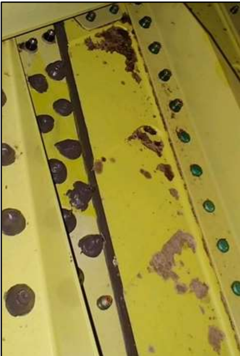
Figure 2 Areas of typical microbiological growth on the lower surface of a wing tank
